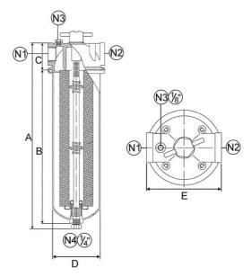
N1: Inlet, N2:Outlet, N3: Vent, N4: Drain
