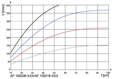
The curves indicate the vclume flow through the complete filter system (filter housing including element) and are referred to a differential pressure of 0.3 bar. Specific process information is essential to guarantee reliable operation of an automatic filter.
