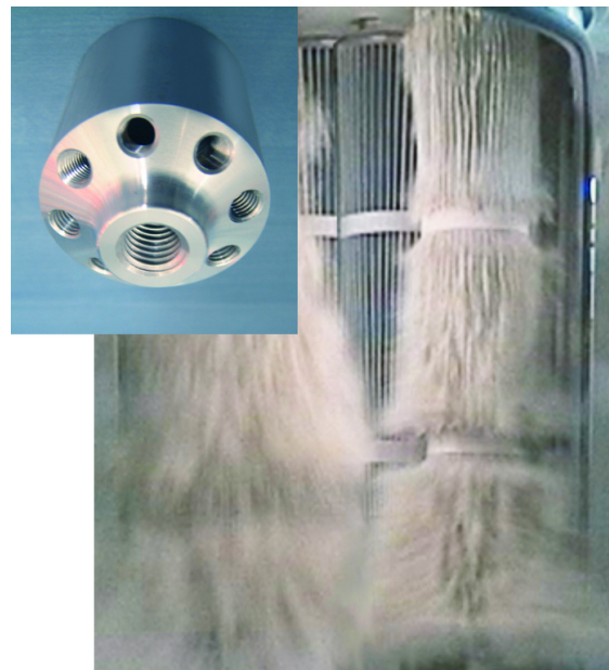
Multi-jet nozzle during cleaning
