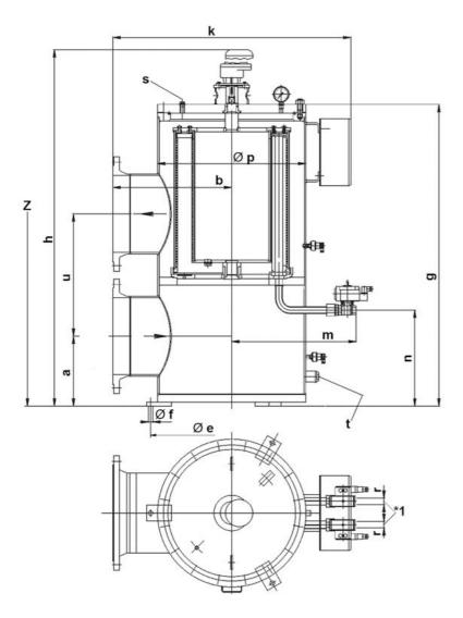
t = Drain s = Vent Z = Clearance required\*1 = Flush pipe
