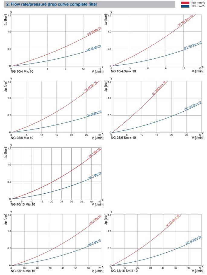
x = flow rate V [l/min]
